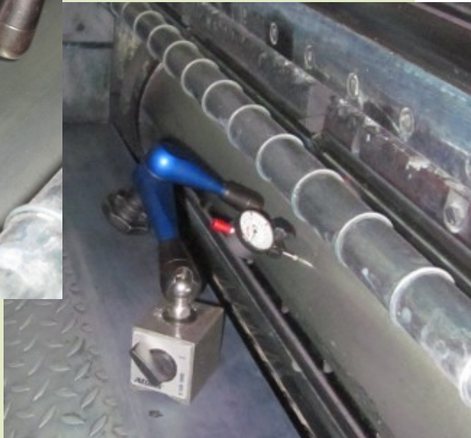
Checking the concentricity of the cylinder
